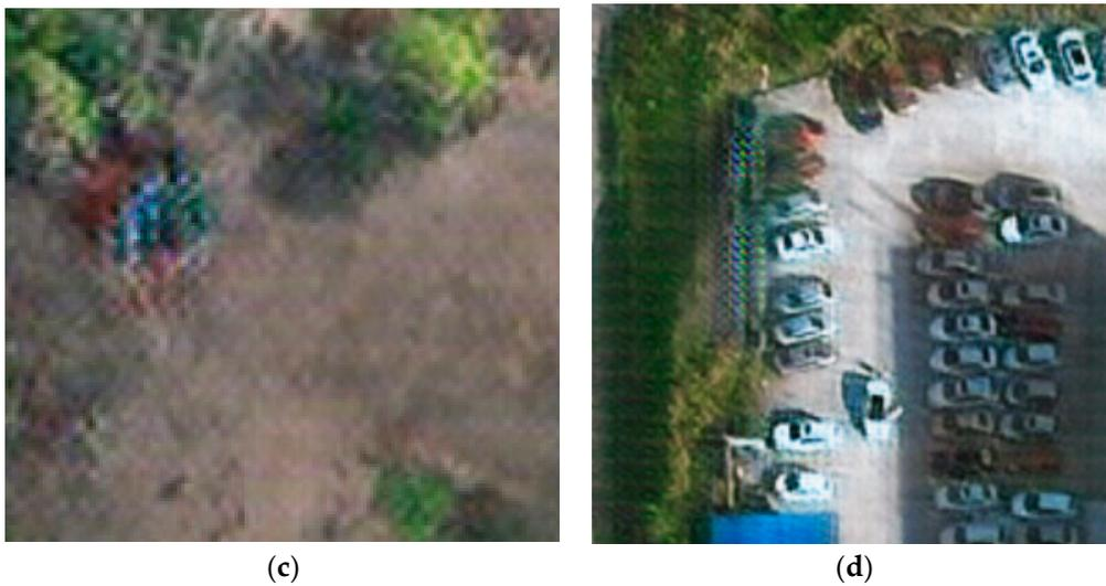
**Figure 3.** An example of “checkerboard artifacts” in the generated photography: (a) input photography; (b) parts of artifacts in generated photography; (c,d) are enlarged parts of (b) where artifacts are obvious.
