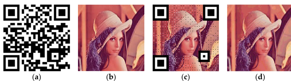
Figure 2. (a) the generated QR code (b) original image (c) image-based QR code (d) the recovered image.
