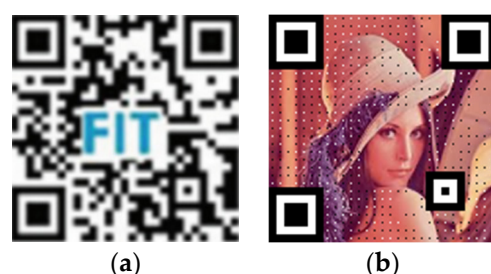
Figure 11. The generated image-based QR code by (a) Wakahara et al. [13] and (b) the proposed method.
