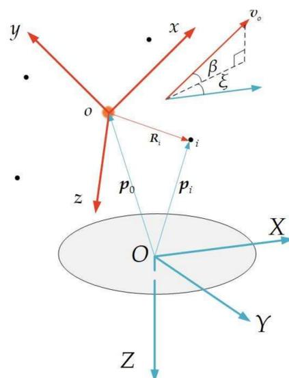
Figure 1. The positional relationships of two coordinate systems.
