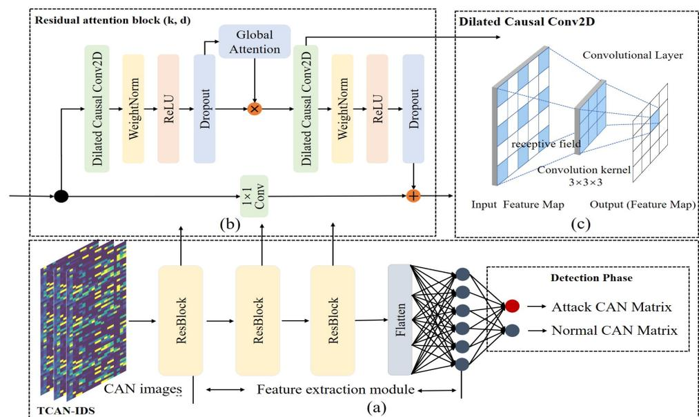
**Figure 3.** The structure of TCAN-IDS: (a) The two stages of feature extraction and detection performed by IDS on the input CAN image. (b) The detailed structure of the residuals in the feature extraction module. (c) The working model of the null convolution in the residual structure.
