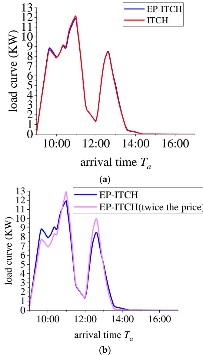
**Figure 11.** Load profiles under different tariffs in the ITCH model and the EP-ITCH model. (a) The comparison of load curves between EP-ITCH model and ITCH model under default the prices. (b) The comparison of the load curves of the EP-ITCH model under default the prices and double the prices.
