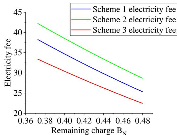
Figure 8.  $T_a = 9:00$ , the trend in electricity fee varies with  $B_N$ .
