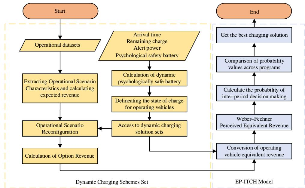
**Figure 1.** EP-ITCH charging model based on WFL.
