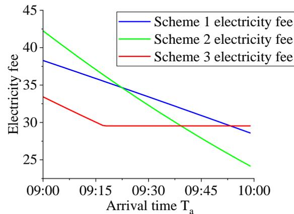
Figure 7.  $B_N = 0.37227$ , the trend in electricity fee varies with  $T_a$ .
