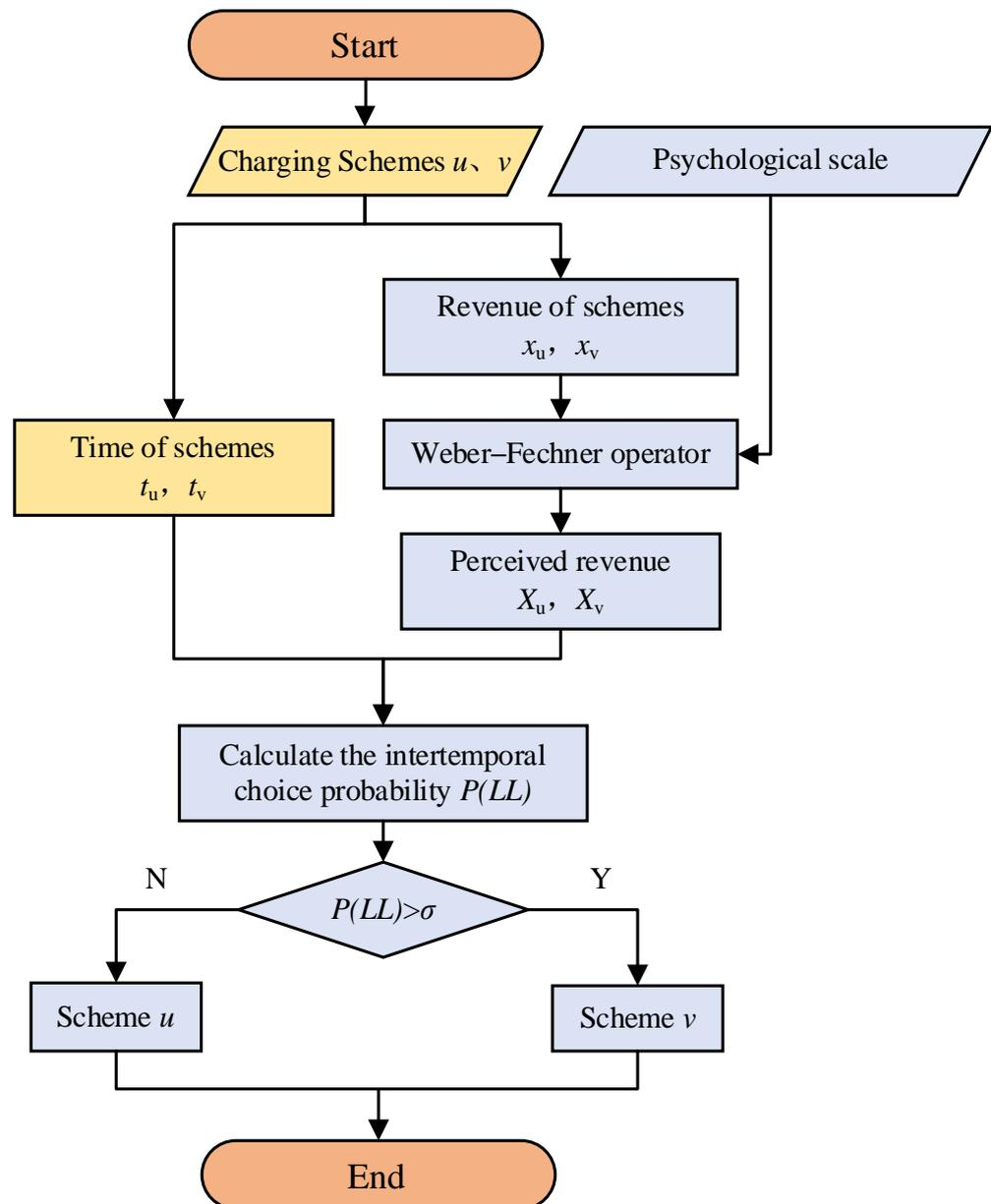
**Figure 4.** Flowchart of the Weber–Fechner-based EP-ITCH charging model.
