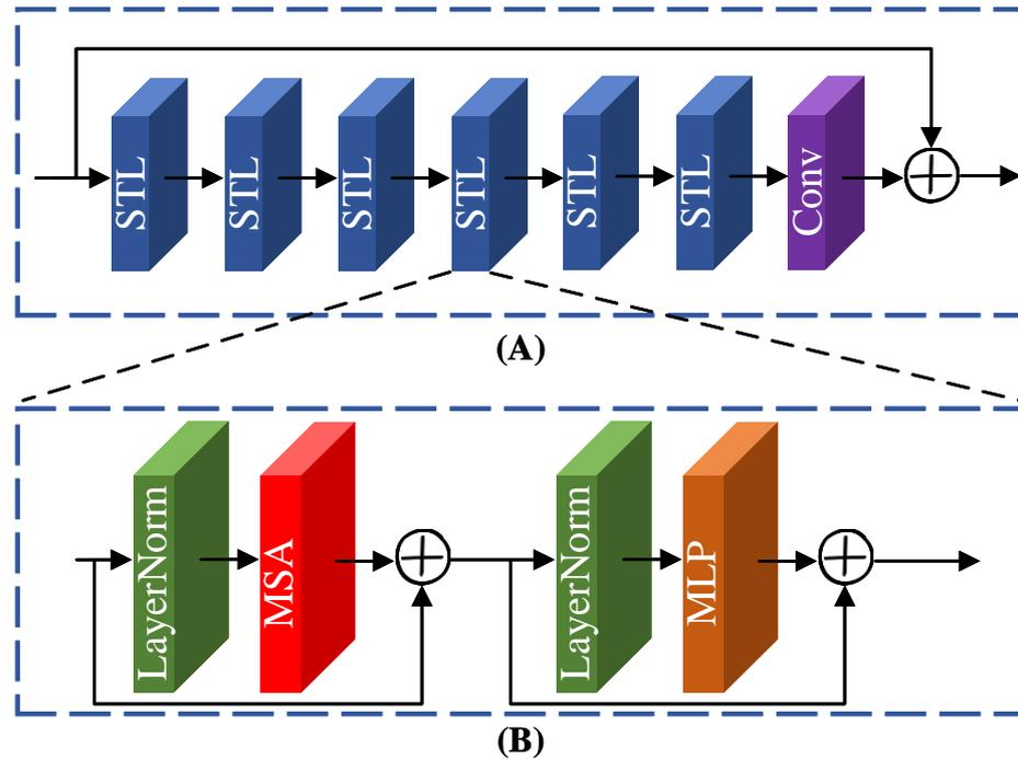
**Figure 5.** The architecture of RSTB. (A) Shows the overall structure of an RSTB, which contains six Swin Transformer layers (STLs) and one convolution layer. (B) Shows the detailed structure of an STL.
