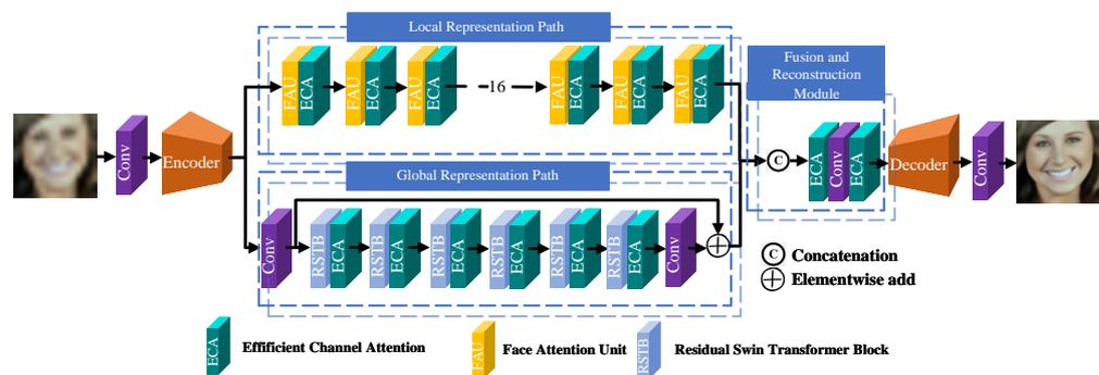
**Figure 2.** The overall architecture of SwinDPSR, which consists of five components: encoder, global representation path composed of RSTB, local representation path composed of Facial Attention Units (FAUs), fusion and reconstruction module (FRM), and decoder.
