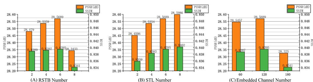
Figure 8. Ablation experiments with different numbers of RSTBs, STLs, and embedded channels.
