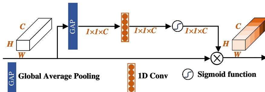
Figure 6. ECA module structure diagram.
