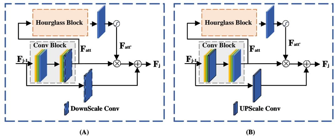
**Figure 4.** The architecture of encoder and decoder: (A) shows the detailed structure of encoder; (B) shows the detailed structure of decoder.
