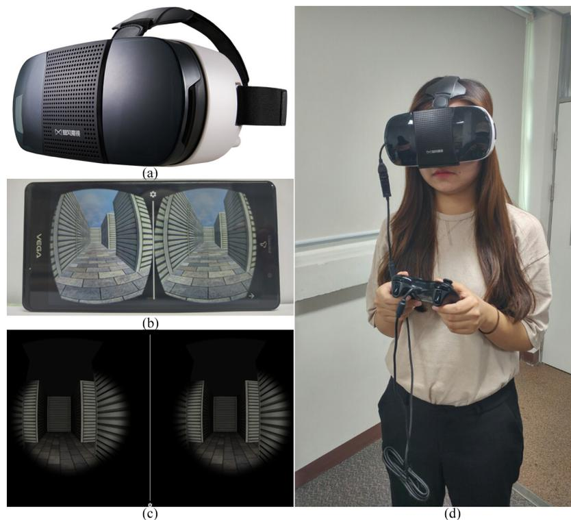
**Figure 11.** Experience environment of the contents using the proposed maze space: (a) mobile HMD (Head Mounted Display) used in the experiment; (b) operation outcome of the mobile virtual reality contents; (c) actual maze scene used in the experiment; and (d) users' experience.
