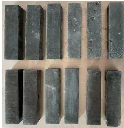
**Figure 3.** Test specimens of flexural and compressive strength of geopolymer.
