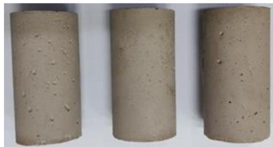
**Figure 4.** Cemented tailings backfill specimens.
