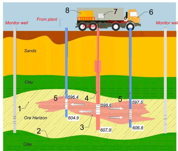
**Figure 4.** Scheme for the intensification of downhole uranium production 1—productive horizon; 2—impenetrable rocks; 3—sedimentation in the NFZ; 4—pumping wells; 5—injection wells; 6—equipment for chemical treatments; 7—pressure hose; 8—tank.
