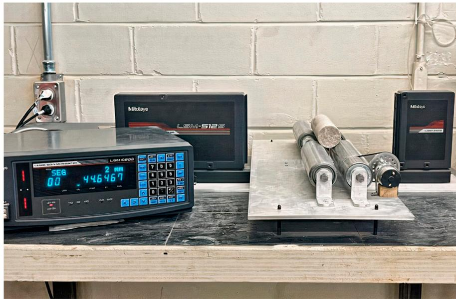
Figure 5. Measurement apparatus of diametrical core deformation.
