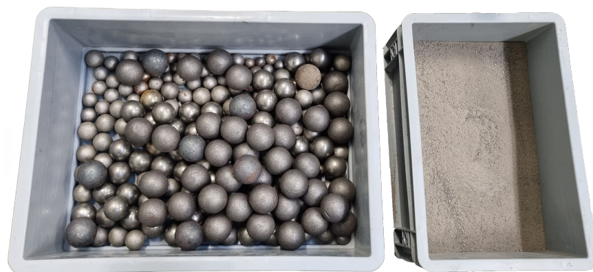
Figure 6. Sample ball and ore load.
