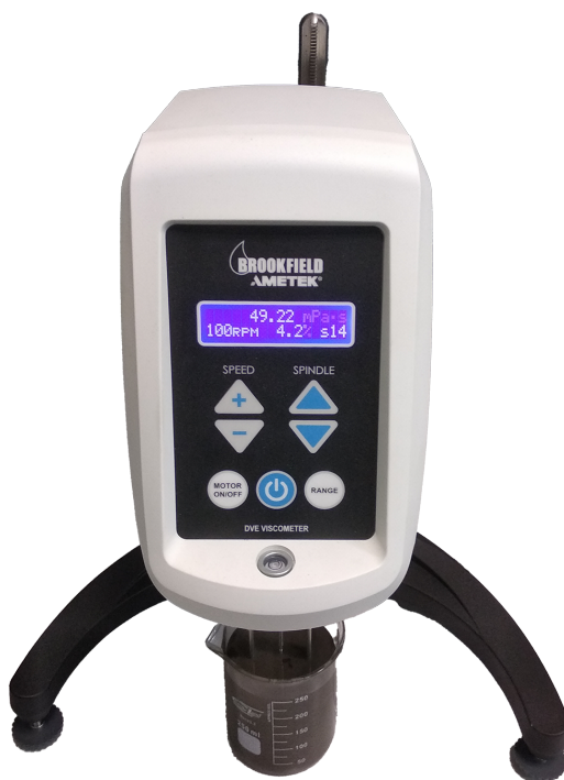
Figure 5. Viscosity measurement of copper ore slurry.
