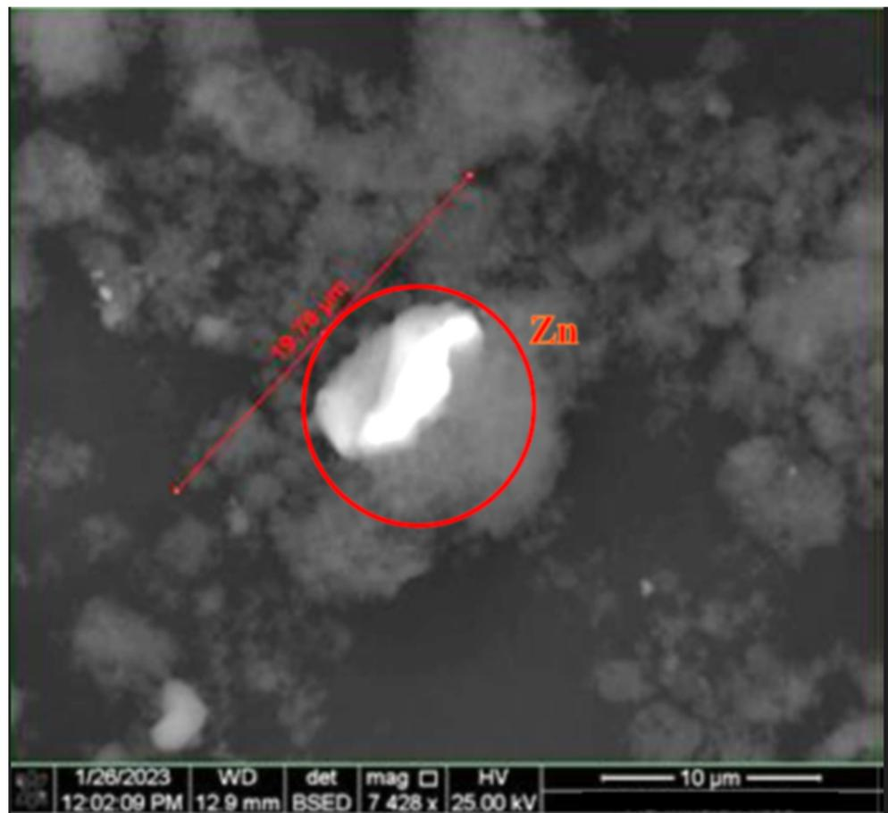
**Figure 10.** Punctual analysis of clots formed in electrocoagulation of 8 L of mining unit water, using aluminum electrodes, magnified at 7428×, resulting in the trapped zinc.
