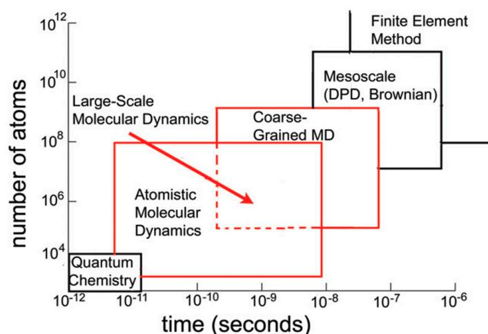
Electronic structure methods such as Hartree-Fock and density functional theory (DFT) include electronic effects (*i.e.*, electron transfer, bond breaking/forming, UV spectroscopy) and represent the highest level of theory, firmly based in quantum mechanics (QM), which can be applied to chemical systems. However, owing to the high computational cost of such methods, their use on NOM or
