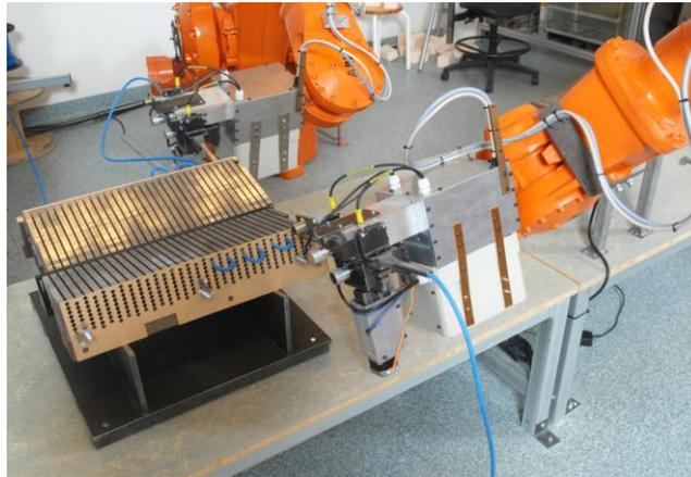
**Figure 5.** (a) A proximity sensor was mounted on top of a cable feeder robot tool and used to take positional measurements on the stator section. (b) The three Tool Centre Point Coordinate Systems (TCPCSs) created at the cable feeder tool and used for positioning the robot. One TCPCS is placed at the sensing distance from the detecting surface of the proximity sensor and two are placed on the ends of the cable guiding tubes.
