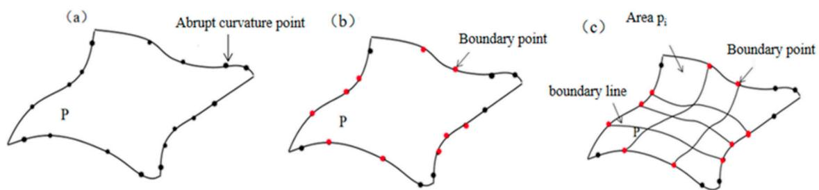
**Figure 1.** Selection of boundary points and region division of surfaces: (a) distribution of abrupt curvature points, (b) selection of boundary points, (c) surface region division.
