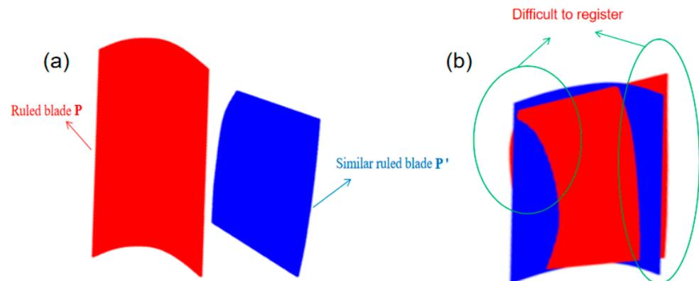
**Figure 5.** Overall point cloud registration of similar surfaces: (a) Point cloud initial state, (b) point cloud overall registration effect.
