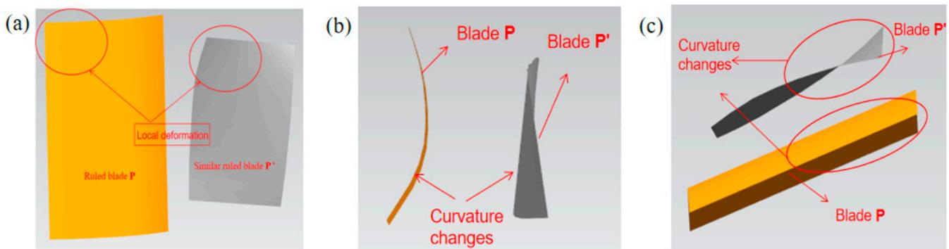
**Figure 4.** Three-dimensional model of two similar blades: (a) local deformation of similar blades, (b) vertical view of similar blades, (c) side view of similar blades.
