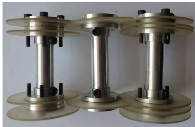
**Figure 3.** Pipeline robot with 2, 4, and 6 bowls.
