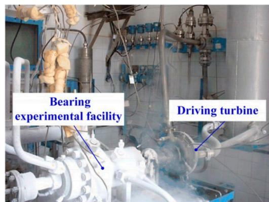
Figure 21. Ultra-low temperature ball bearing testing machine.
