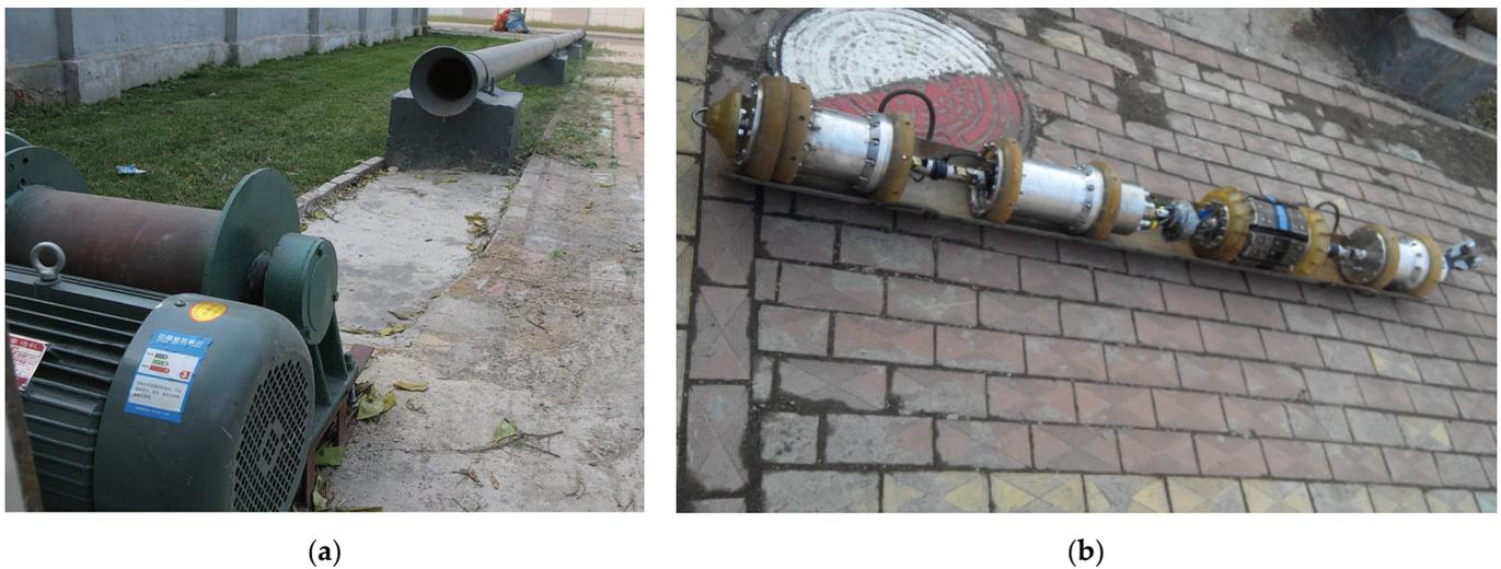
**Figure 7.** Photos of the test field and MFL internal detector. (a) The traction test field; (b) The MFL internal detector.
