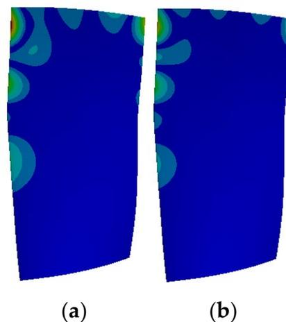
**Figure 24.** 54 EO displacement amplitude of R1 rotor blade. (a) C# (b) M#.
