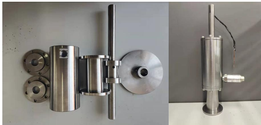
**Figure 25.** Prototype of double-rod magnetorheological damper.
