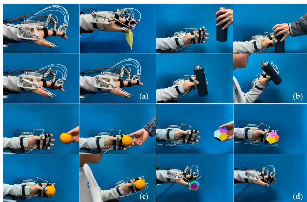
**Figure 15.** Grasp ability experiment: (a) Pinching paper; (b) Grasping a cup; (c) Picking an orange; (d) Handling a Rubik's cube.
