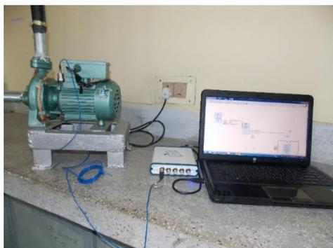
Figure 10. Centrifugal pump test bench.
