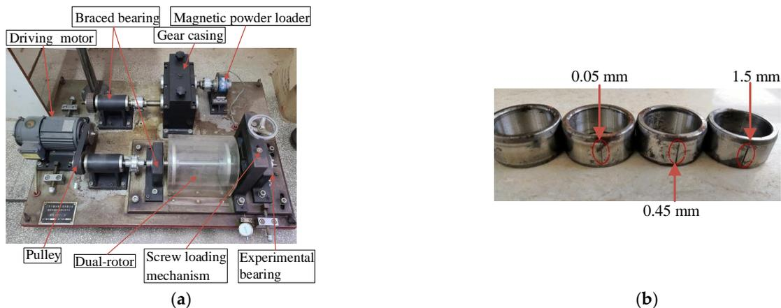
**Figure 5.** Experimental platform: (a) The test bench; (b) photographs of defective components under study.
