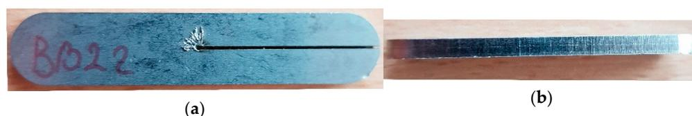
**Figure 2.** AISI 304 stainless-steel specimen obtained after laser cutting: (a) top view; (b) side view.
