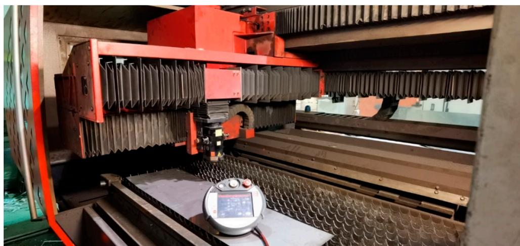
**Figure 1.** CO<sub>2</sub> laser cutting machine used in the experiment.
