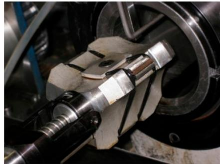
**Figure 3.** Honing head provided with cBN abrasive stones.
