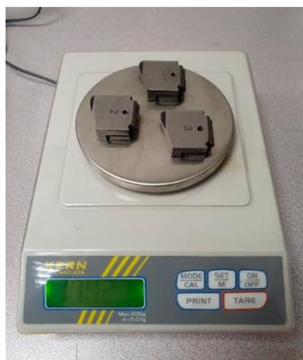
**Figure 5.** Scale used to weigh the abrasive stones and tool holders.
