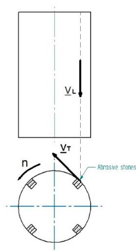
**Figure 1.** Schematic of the honing process:  $V_L$  is linear speed of the honing head,  $V_T$  is tangential speed (corresponding to the rotation speed  $n$  of the cylinder). In this example, the honing head is provided with 4 abrasive stones.
