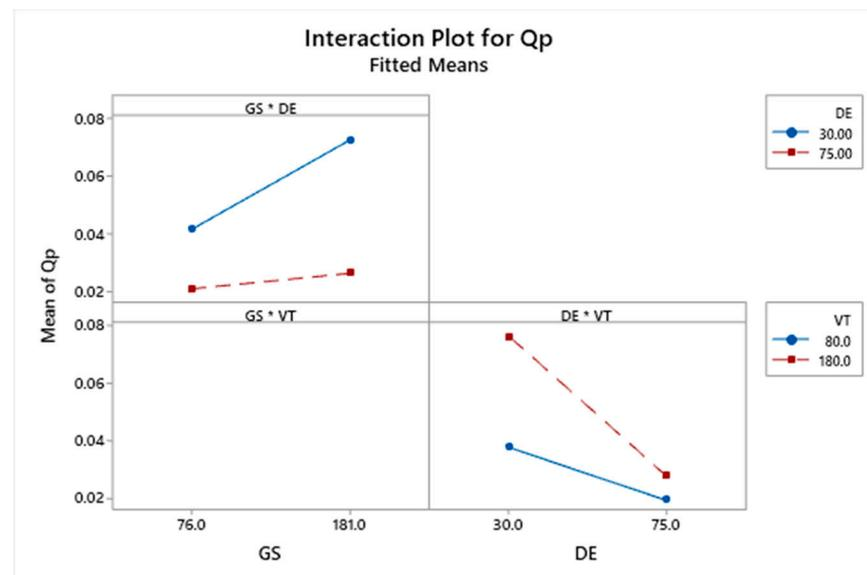
Figure 10. Interaction plot for tool wear  $Q_p$ .
