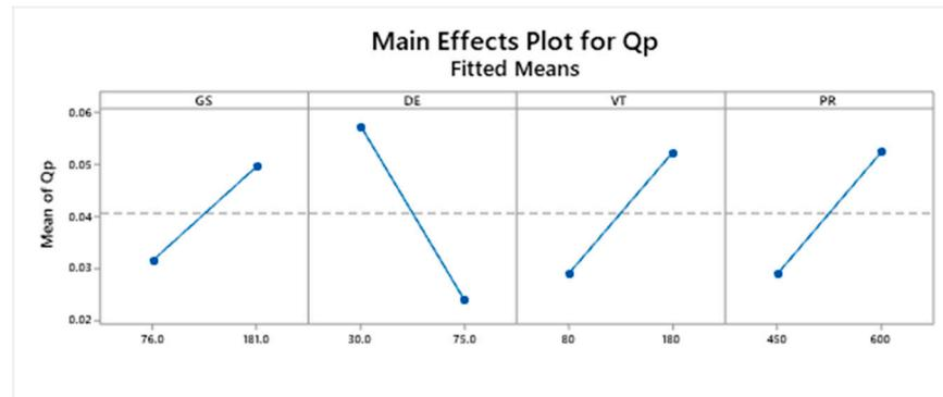
Figure 9. Main effects plot for tool wear  $Q_p$ .
