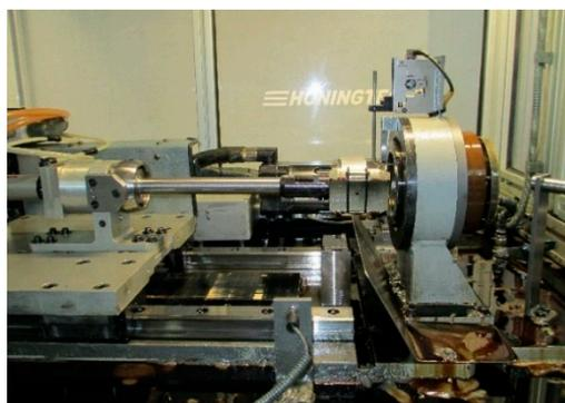
Figure 2. Honing test machine.
