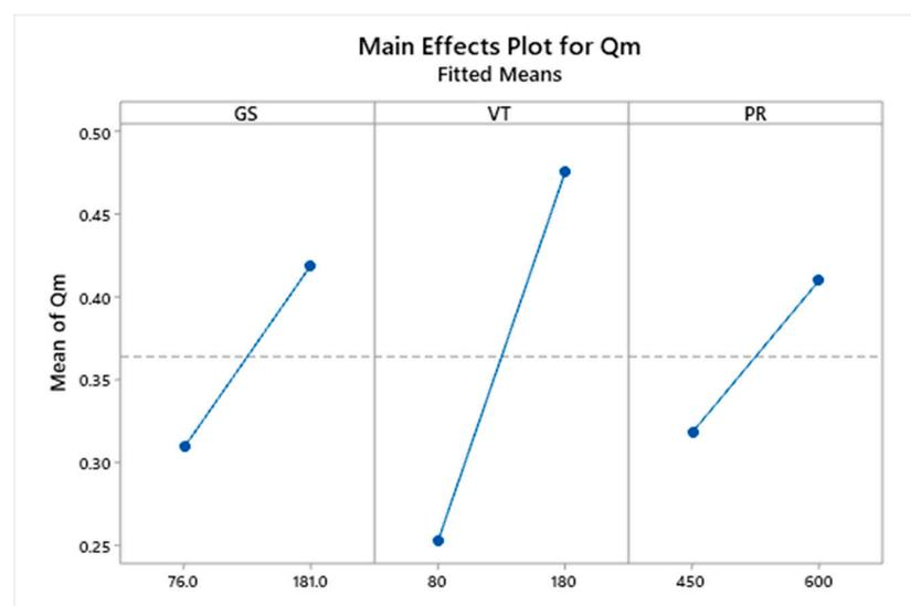
**Figure 6.** Main effects plot for material removal rate Qm.
