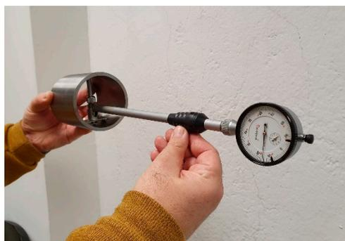
**Figure 4.** Alexometer used to measure the internal diameter of the cylinders.
