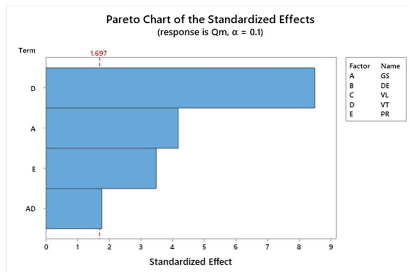
Figure 8. Pareto chart of the standardized effects for material removal rate  $Q_m$ .
