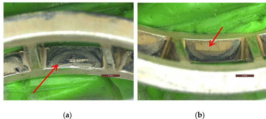
Figure 15. Contact wear morphologies of the side beams, as the arrow indicated: (a) wear of the side beam, corresponded to the bearing side with laser marking; (b) wear of the other side beam.
