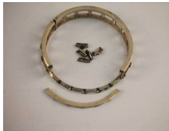
Figure 13. Macroscopic damage morphology of the cage.
