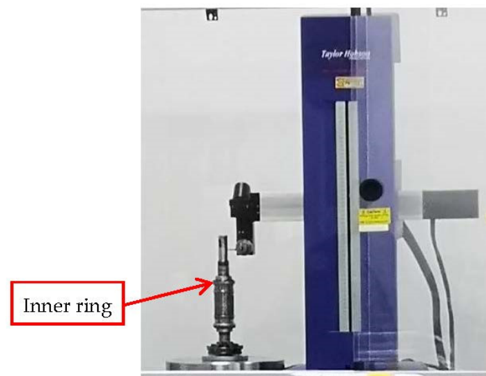
Figure 18. Cylindricity of the inner ring fixed on the shaft is to be measured.
