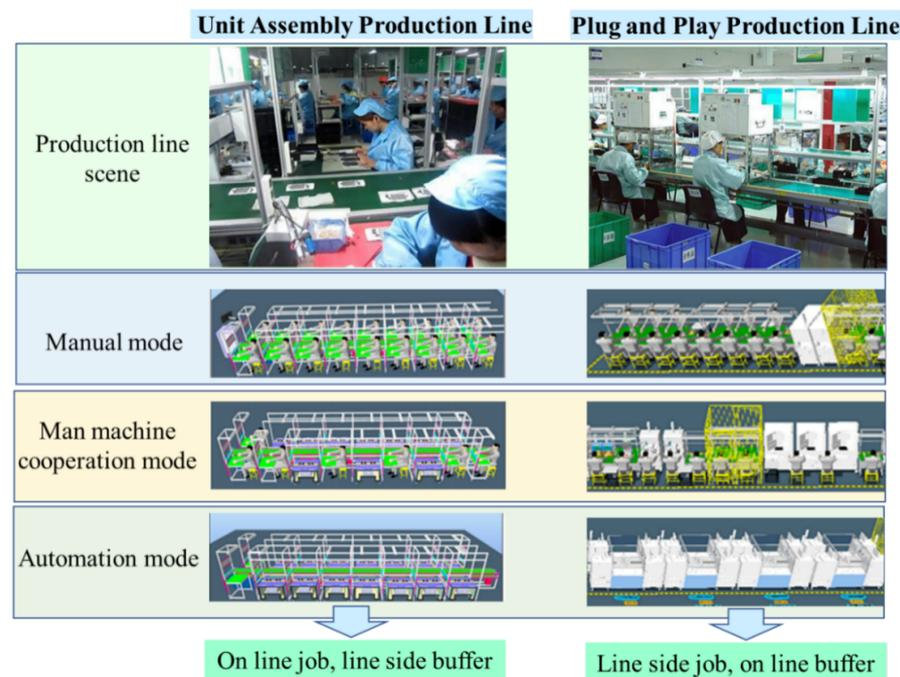
Figure 3. Comparison of two production line architecture forms.
