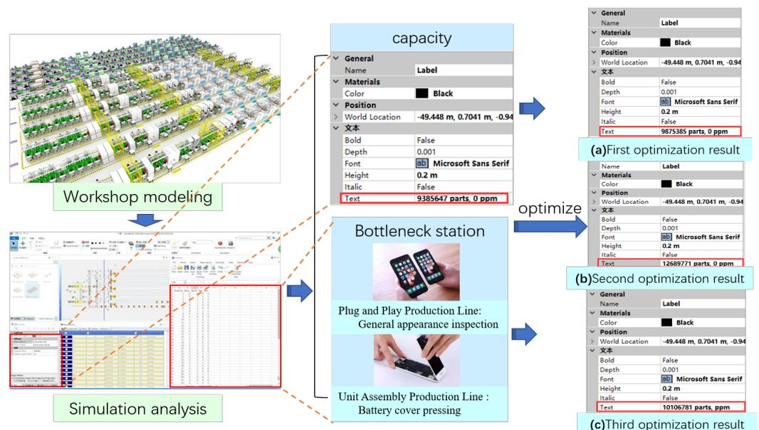
**Figure 7.** Simulation and optimization of workshop. (a) The results of optimization of all unit assembly lines in the workshop. (b) The result of optimization of all plug and play assembly lines and unit assembly lines simultaneously. (c) The result of iterative optimization.
