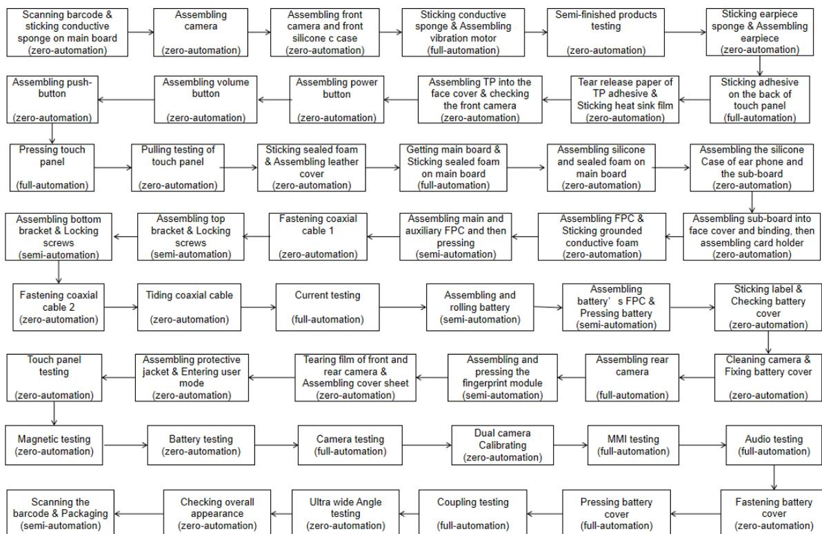
Figure 2. Station division and automatic analysis of a certain type of mobile phone.
