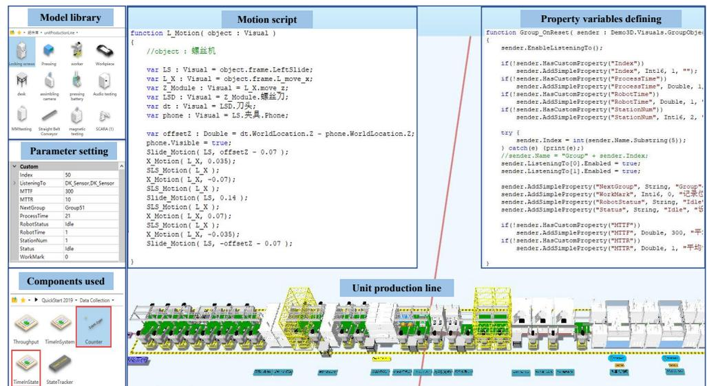
Figure 6. The construction steps of the semi-physical simulation model.
