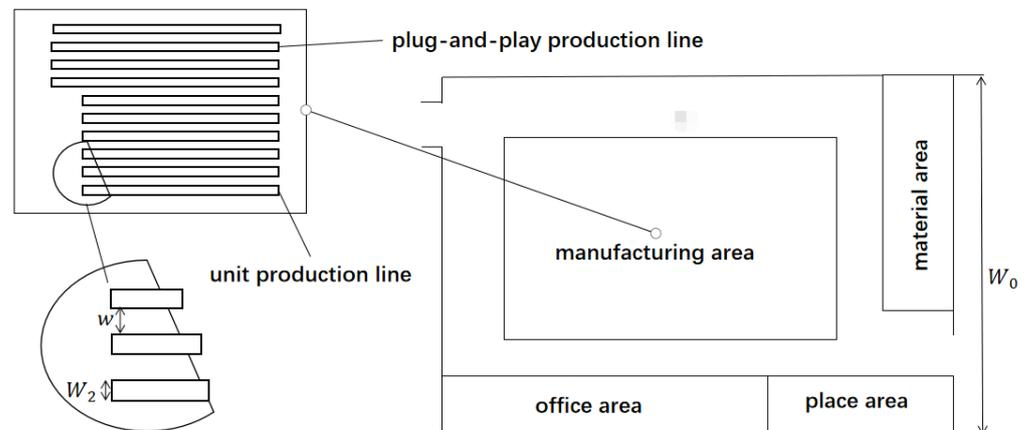
**Figure 5.** The layout of the whole hybrid workshop.
