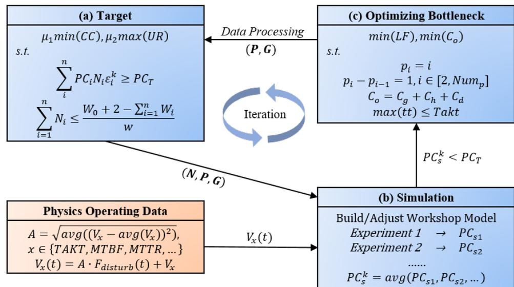
**Figure 9.** The iterative calculation process. (a) The calculation process of related parameters of each type of production line. (b) The process of simulating multiple times. (c) The calculation process of bottleneck optimization.
