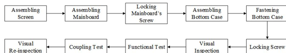
**Figure 1.** Assembly Process of Mobile Phone.
