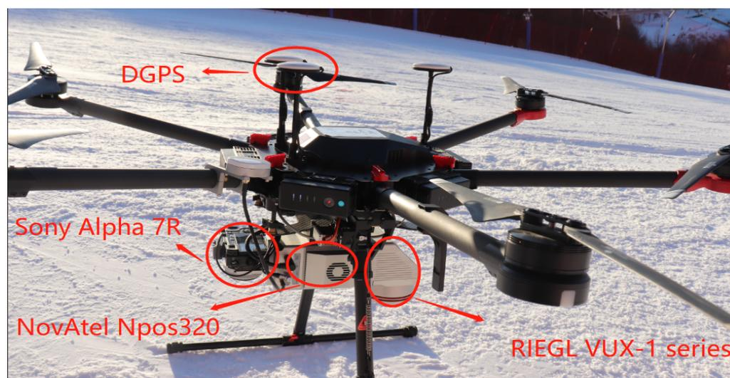
**Figure 2.** Structure diagram of point cloud acquisition system, which mainly includes inertial navigation, DGPS, camera and laser scanning.
