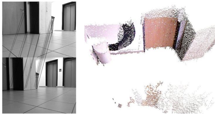
**Figure 3.** Visualized results for the 3D feature matching, and the reconstructed environment.
