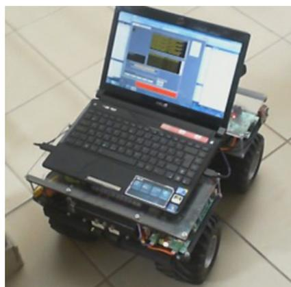
**Figure 1.** The mobile robot built and used for experiments. The experimental setup contains ultrasonic sensors and a commercially available Kinect sensor.
