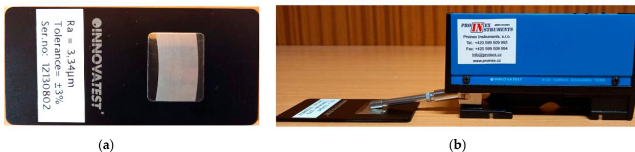
**Figure 4.** (a) Specimen measured to determine roughness parameters; (b) R130 roughness tester at work.
