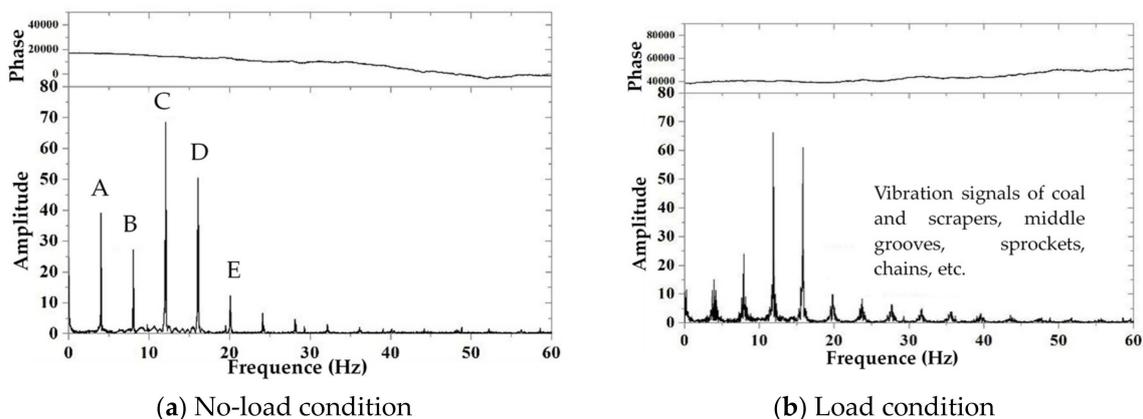
Figure 13. Spectrograms of vibration signals under no-load and load conditions.
