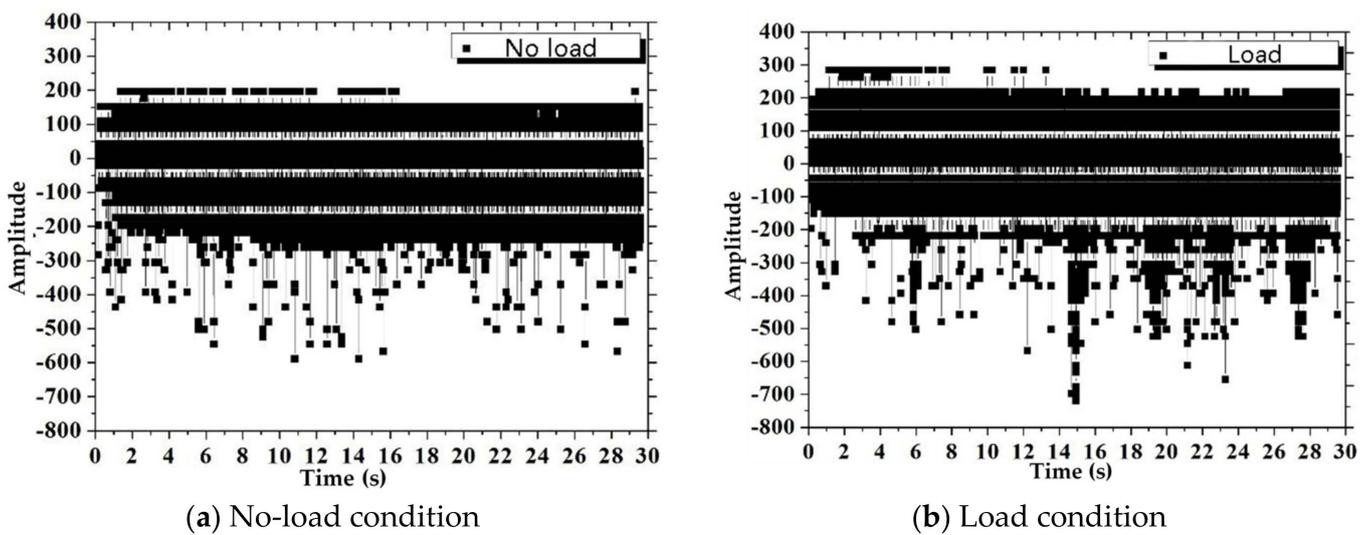
**Figure 11.** Vibration signals under no-load and load conditions.
