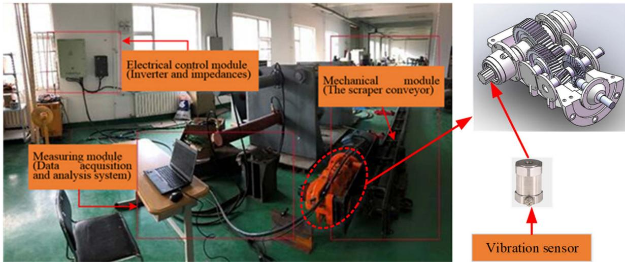
Figure 1. Test bench of dynamic properties for the scraper conveyor.
