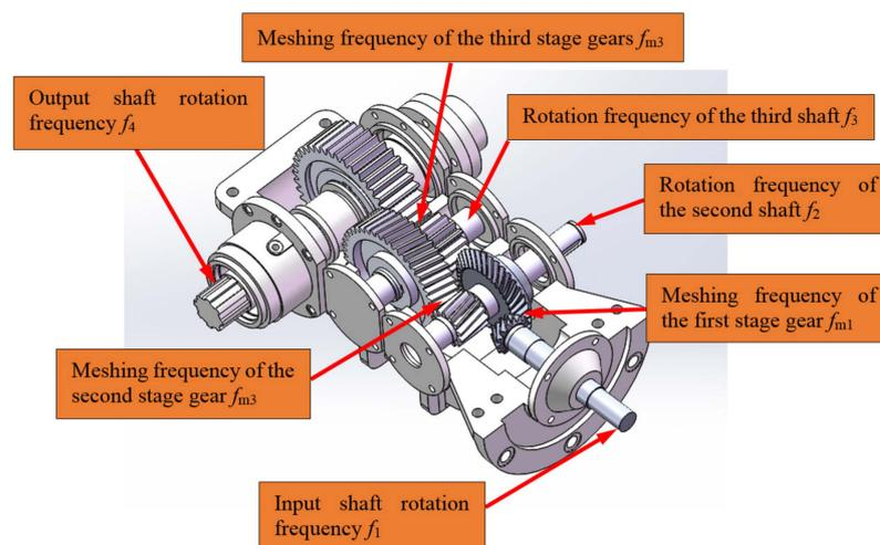
Figure 5. Three gear transmissions in the gear reducer.
