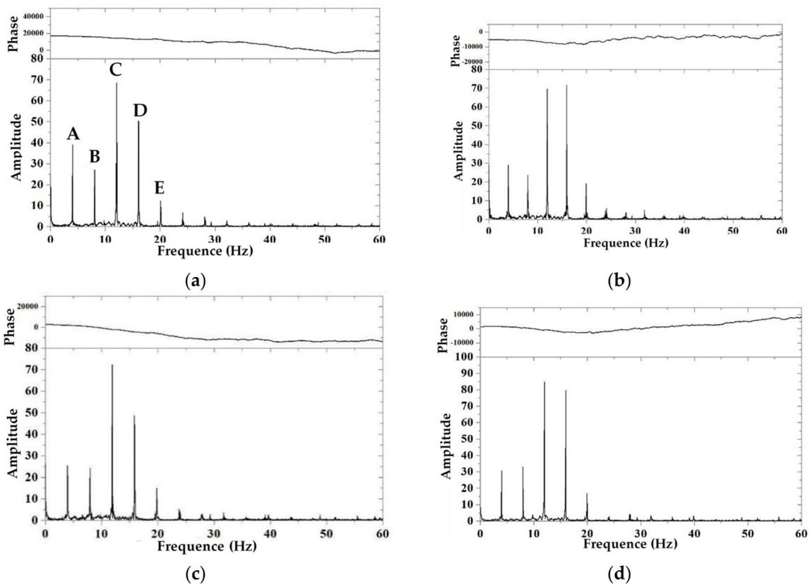
**Figure 10.** Spectrograms of vibration signals under four various terrain conditions. (a) Straight working condition. (b) Horizontal bending condition. (c) Vertical bending condition. (d) Combined working condition of horizontal and vertical bending.
