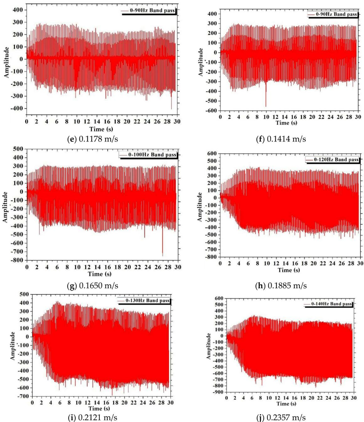
**Figure 6.** Vibration signals of 10 groups under different chain speeds.
