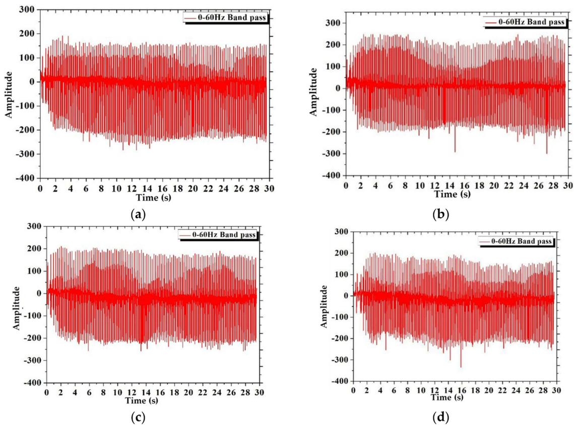
**Figure 9.** Vibration signals under four various terrain conditions after FFT filtering. (a) Straight working condition. (b) Horizontal bending condition. (c) Vertical bending condition. (d) Combined working condition of horizontal and vertical bending.
