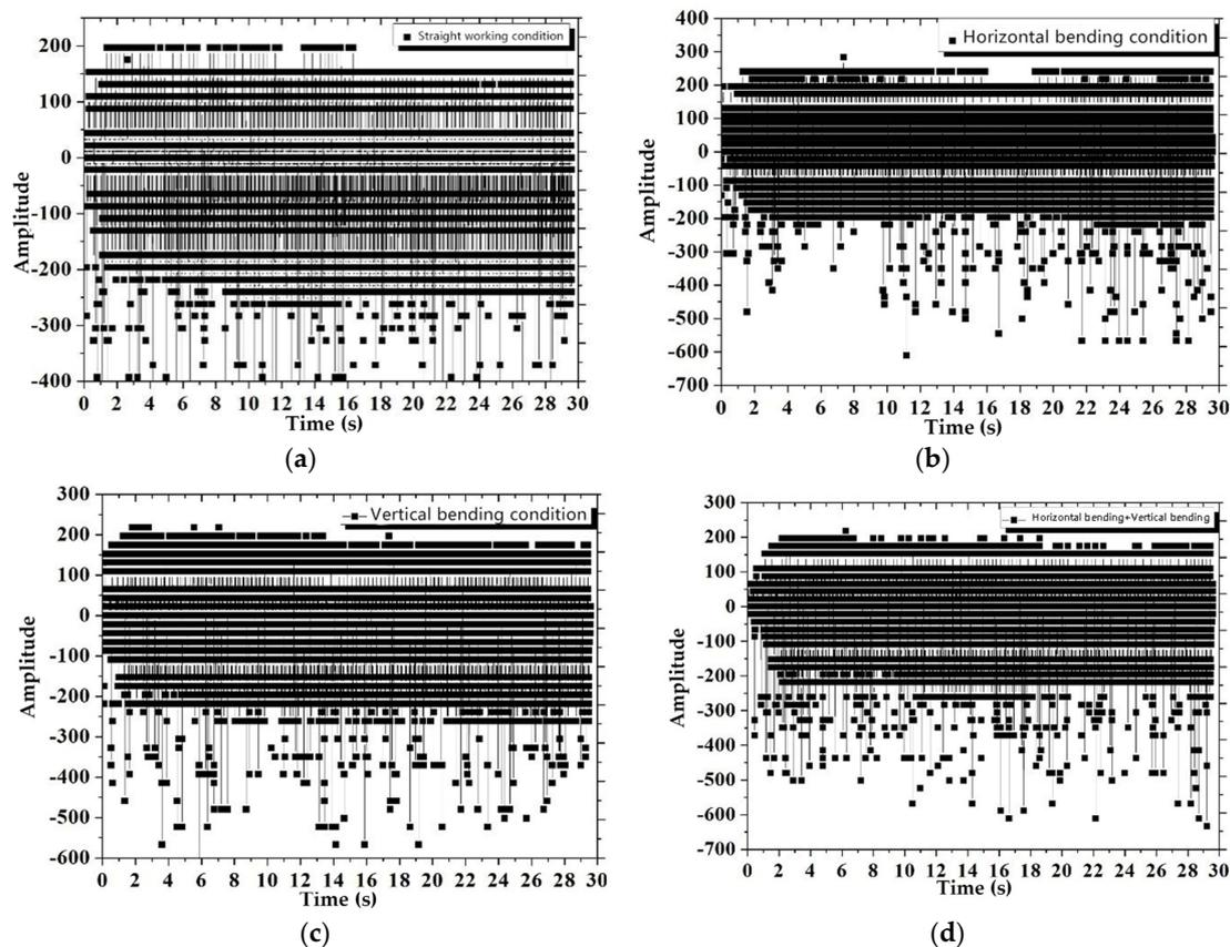
**Figure 8.** Vibration signals under four various terrain conditions. (a) Straight working condition. (b) Horizontal bending condition. (c) Vertical bending condition. (d) Combined working condition of horizontal and vertical bending.
