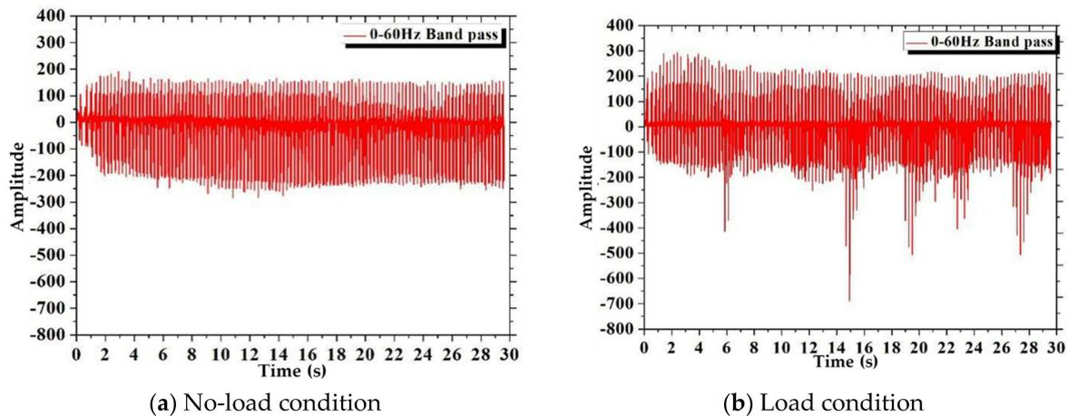
Figure 12. Vibration signals under no-load and load conditions after FFT filtering.
