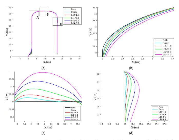
**Figure 13.** Pure tracking algorithm of fuzzy control. (**a**) Bow turn path tracking; (**b**) Partial enlargement at A; (**c**) Partial enlargement at B; (**d**) Partial enlargement at C.
