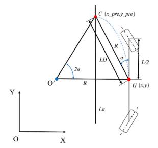
Figure 4. 4WS pure tracking model.
