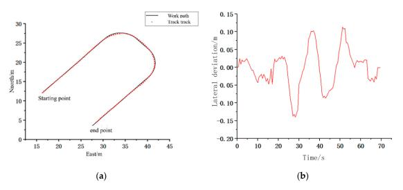
Figure 20. Bow turn route tracking track (a) Bow-turn section path tracking; (b) Lateral deviation.
