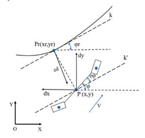
Figure 8. Lateral deviation and heading deviation.
