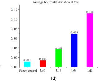
**Figure 15.** Comparison of lateral deviation of bow turn path. (**a**) Peak lateral deviation; (**b**) Average lateral deviation at A; (**c**) Average lateral deviation at B; (**d**) Average lateral deviation at C.
