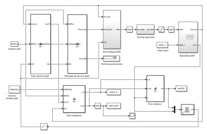
Figure 11. 4WS pure tracking algorithm simulation model.
