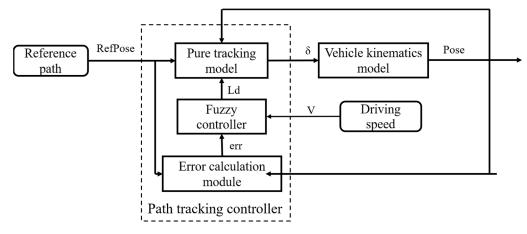
Figure 10. Path tracking simulation flow chart.
