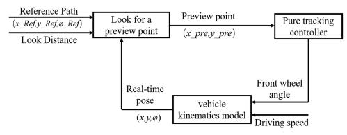
Figure 3. Framework diagram of traditional pure tracking algorithm.
