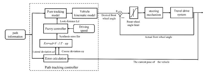
Figure 1. Schematic diagram of the path tracking system.
