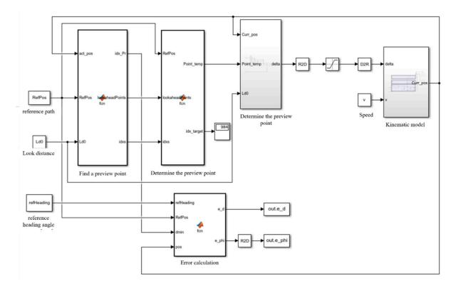
Figure 5. Simulation model of 4WS pure tracking algorithm.
