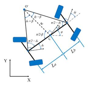
Figure 2. 4WS vehicle kinematics model.
