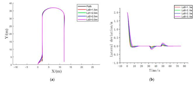
Figure 6. Traditional pure tracking algorithm path tracking. (a) Path tracking curve; (b) Lateral deviation.
