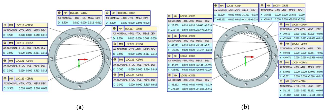
**Figure 2.** The manufacturing errors of the ring gear: (a) the pin-groove radial error; (b) the pin-groove position error.
