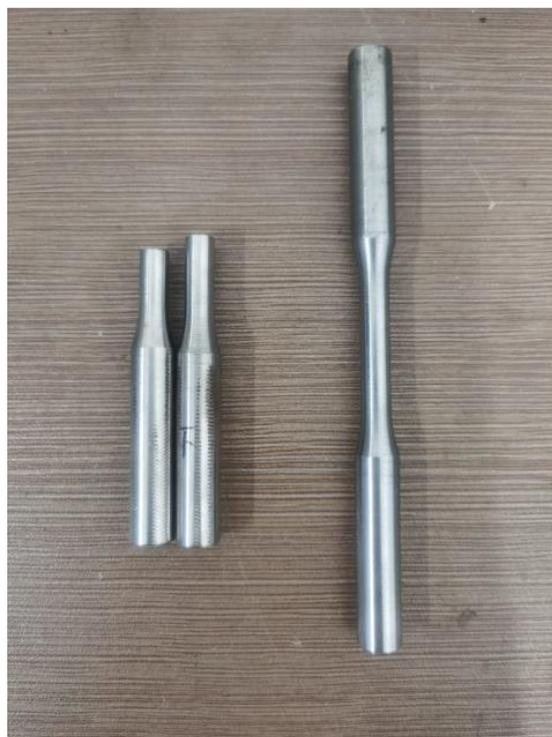
**Figure 5.** Sample rod for fatigue test.
