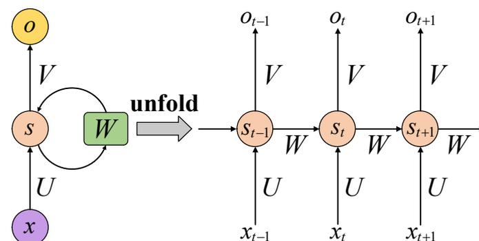
Figure 5. Basic structure diagram of RNN.
