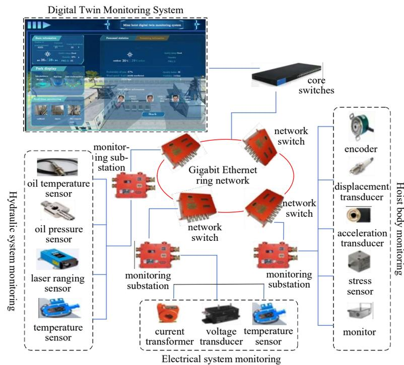
Figure 4. The intelligent sensing network of mine hoist.
