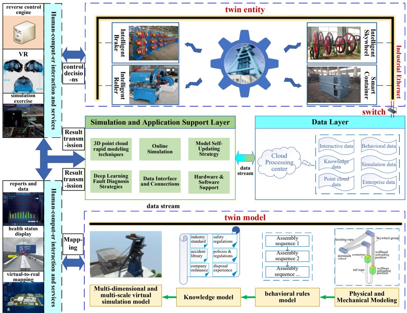
Figure 3. Digital twins structure of mine hoist.
