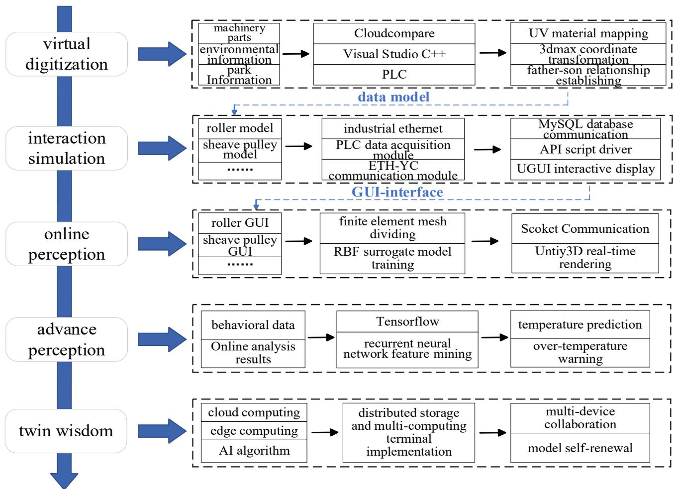
**Figure 1.** Digital twin five-dimensional maturity model of mine hoist.
