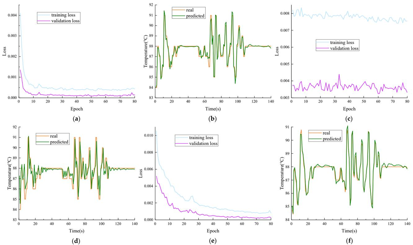
**Figure 10.** Comparison chart of training and prediction results for temperature point sensor 1: (a) loss of LSTM; (b) prediction of LSTM; (c) loss of RNN; (d) prediction of RNN; (e) loss of Gauss–Kalman–LSTM; (f) prediction of Gauss–Kalman–LSTM.
