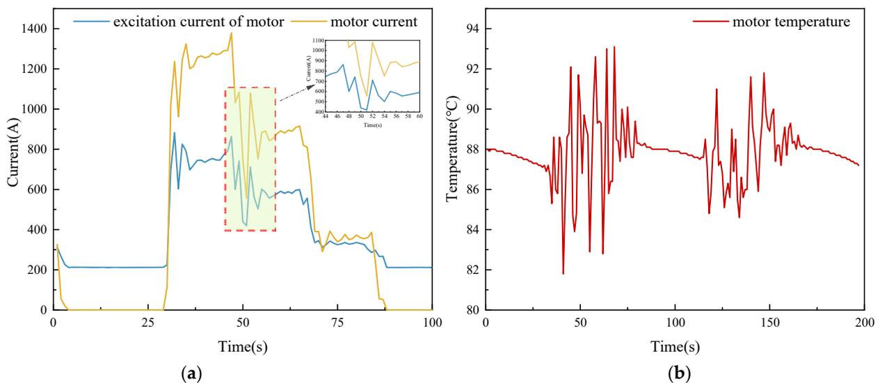
Figure 15. Current and temperature behavioral monitoring of hoist motor: (a) current monitoring; (b) temperature monitoring.
