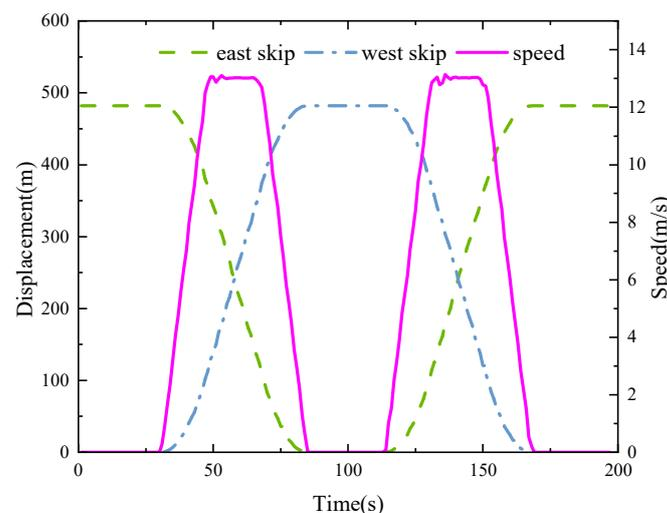
**Figure 13.** Running process diagram of mine hoisting system.
