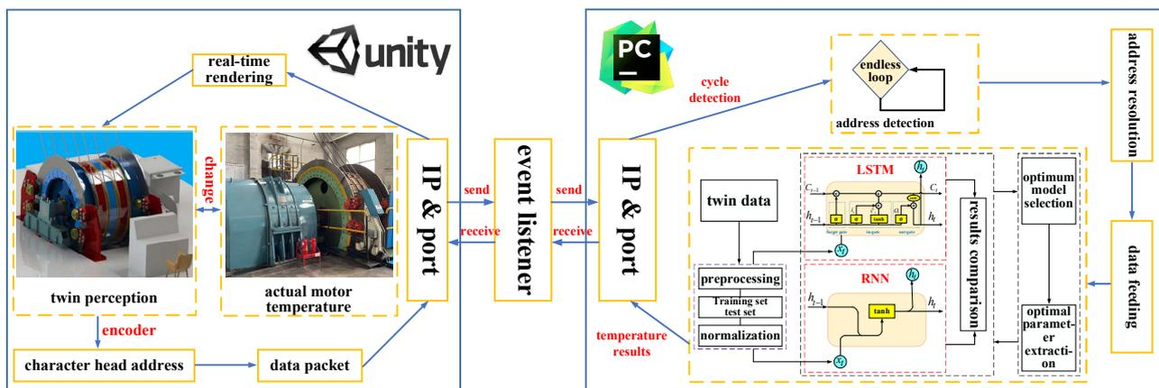
Figure 8. Prediction and sensing flow-chart of hoist based on digital twin.
