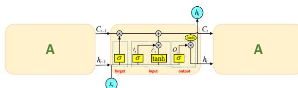
Figure 7. LSTM memory block structure diagram.
