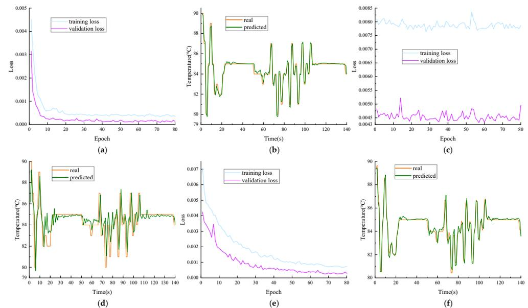
**Figure 12.** Comparison chart of training and prediction results for temperature point sensor 2: (a) loss of LSTM; (b) prediction of LSTM; (c) loss of RNN; (d) prediction of RNN; (e) loss of Gauss–Kalman–LSTM; (f) prediction of Gauss–Kalman–LSTM.
