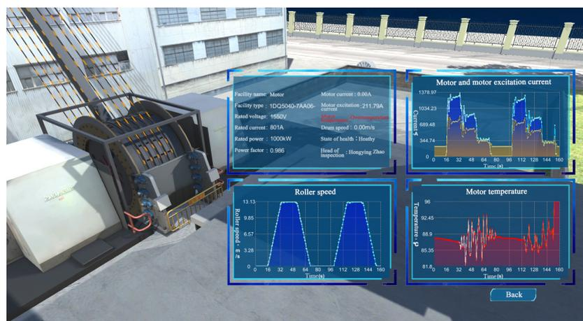
Figure 16. Temperature perception of mine hoist motor in digital twin monitoring system.
