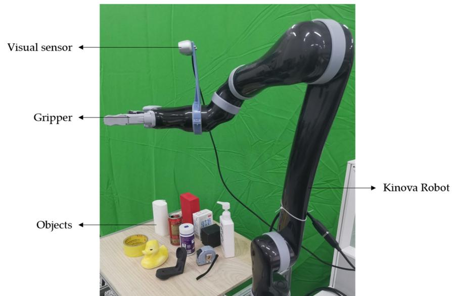
**Figure 8.** The experimental platform for the robot grasping.
