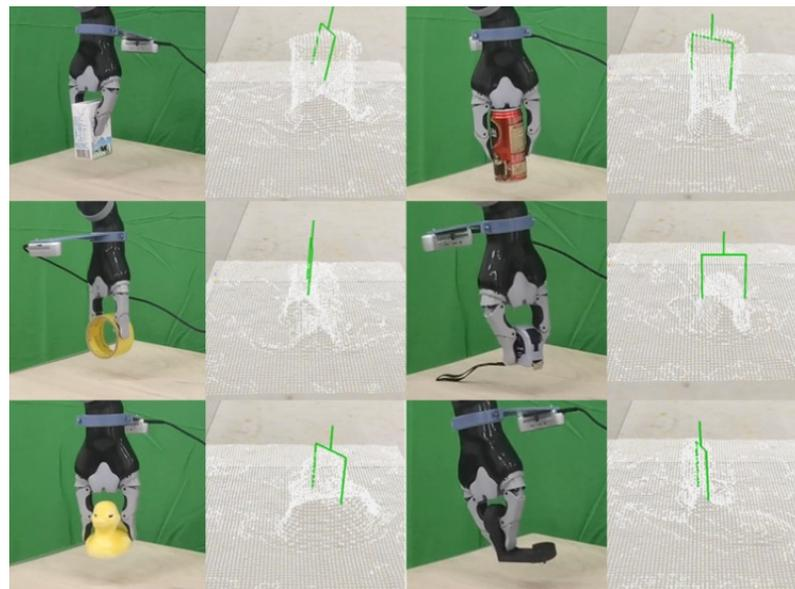
Figure 11. Successful cases in the single-object grasping experiment.
