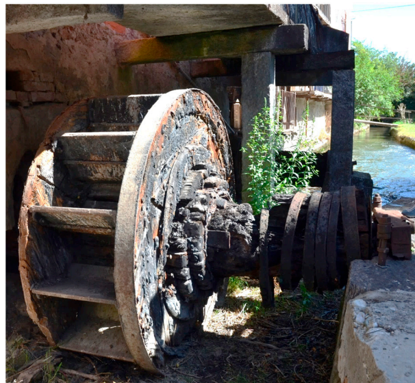
Figure 17. Water wheel #2 powering tilt hammer #2.
