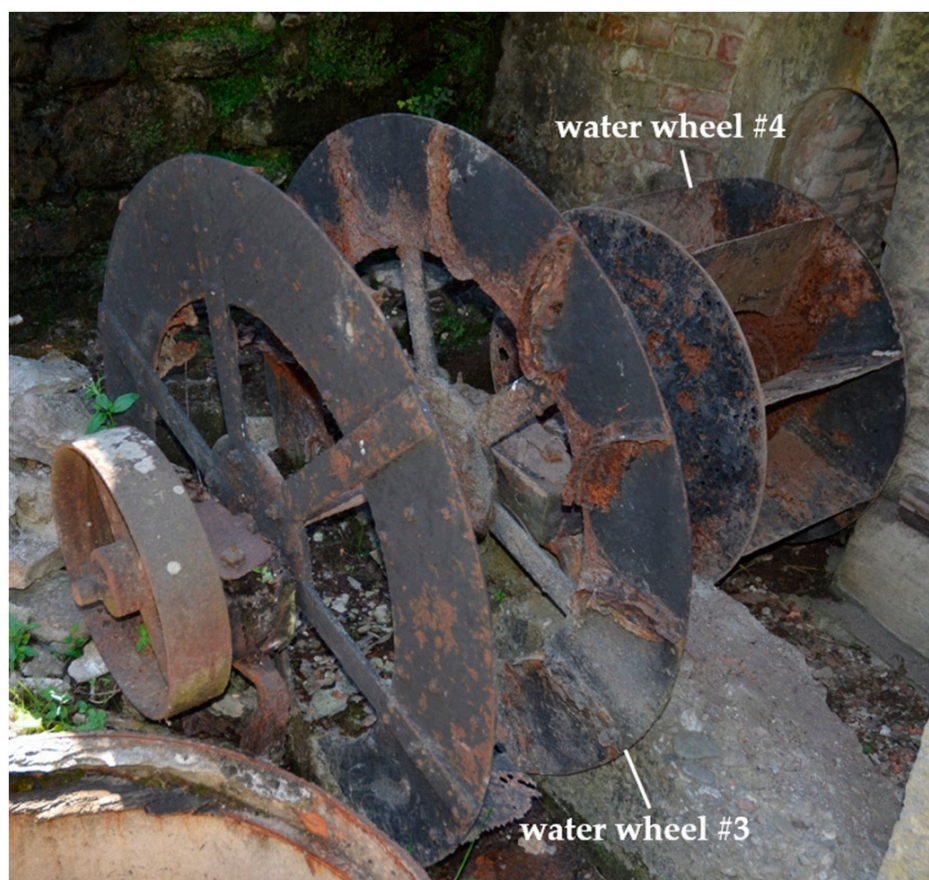
Figure 24. The two water wheels powering the machine tool apparatus.
