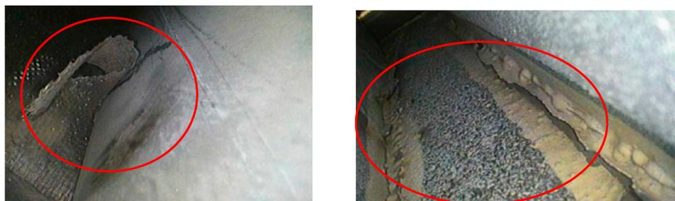
Figure 1. Results from PD activity and electrical stress.
