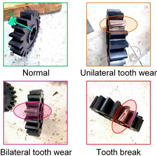
Figure 20. Fault injection of the driving gear.
