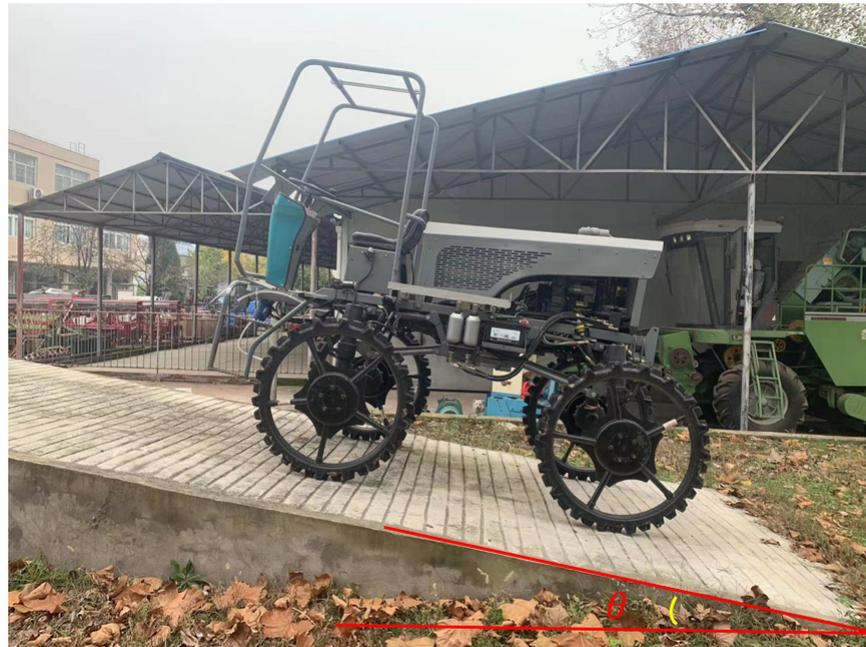
Figure 13. The climbing experiment of HGPM.
