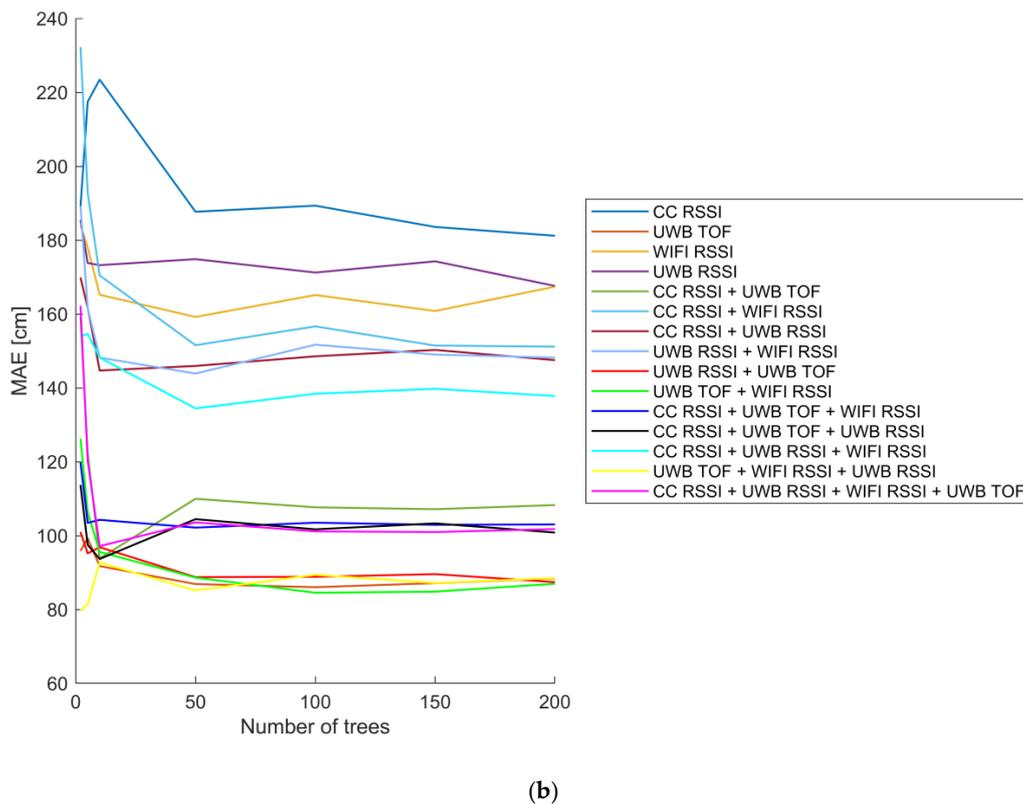
**Figure 8.** The effect of the number of trees: (a) For training data; (b) For test points.
