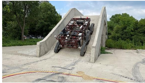
Figure 16. Snapshot of the autonomous controller traversing the slope terrain.
