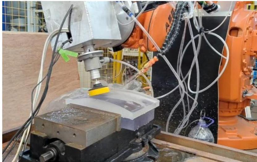
**Figure 11.** Polishing process of the complex curved plexiglass part.
