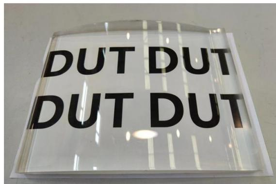
**Figure 14.** The actual effect of the complex curved plexiglass part after polishing.
