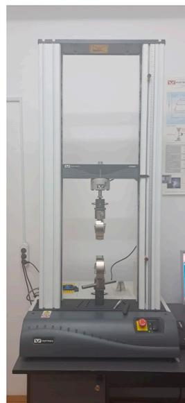
**Figure 4.** Instron 3366 tensile testing machine.
