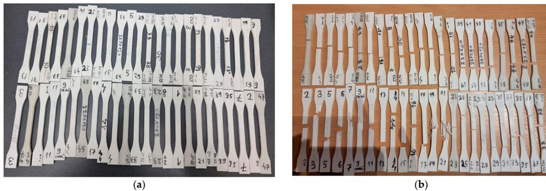
**Figure 3.** Manufactured tensile test specimens (a); test specimens after tensile testing (b).
