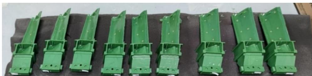
**Figure 5.** Wax patterns of a gas turbine blade.
