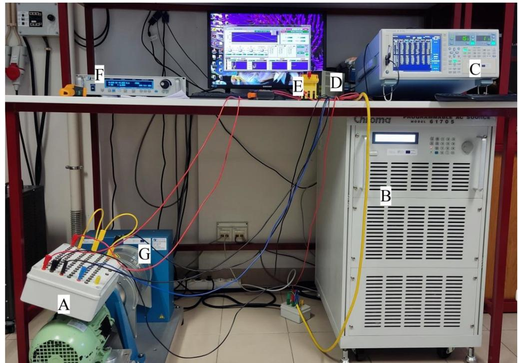
**Figure 4.** LSPMSM test branch. A—LSPMSM, B—Chroma AC Programmable Source, C—YOKOGAWA WT1800, D—Fault resistance, E—Manual switch connected in series with the fault resistance, F—MAGTROL Dynamometer Controller, and G—MAGTROL Hysteresis Dynamometer.
