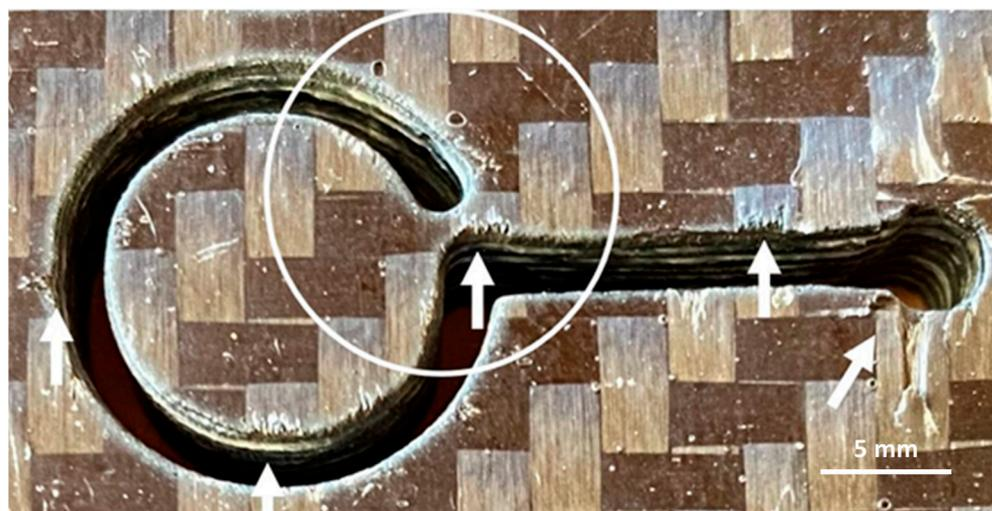
**Figure 5.** Example of surface damage: delamination, fibre pull out, and cavitation (Test 15, top side).
