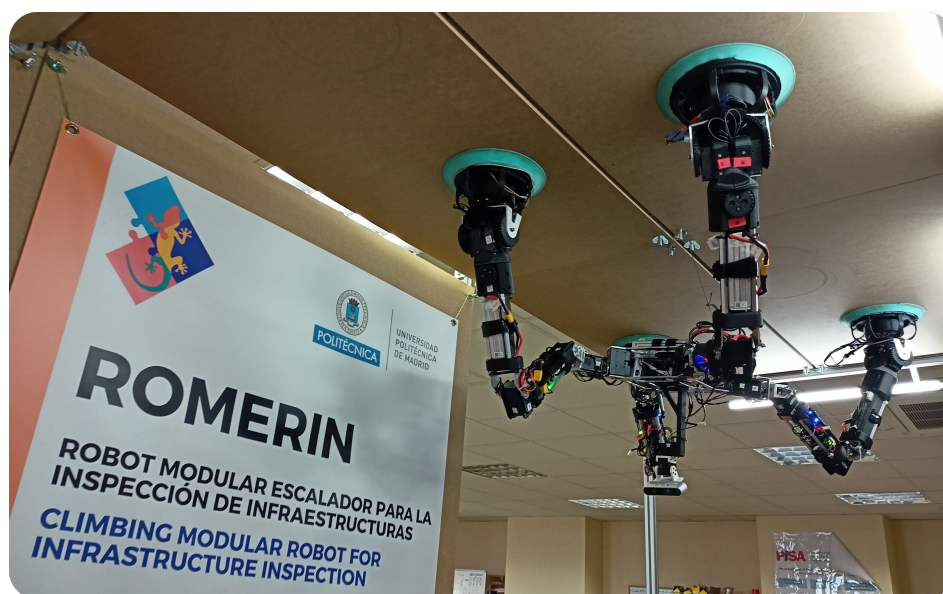
Figure 1. The Romerlin robot fixed to the ceiling of the test bench thanks to its active suction cups.
