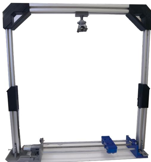
**Figure 4.** Linear Actuator System Artifact.
