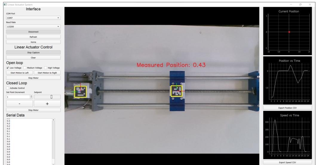
**Figure 23.** Linear Actuator System graphical user interface developed in PyQt5 displaying the cart's measured position in the 2D-plane, and the position and velocity with respect to time.
