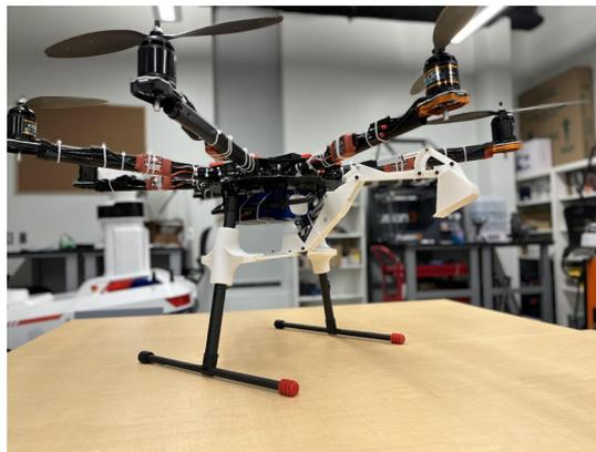
**Figure 2.** The second design of an autonomous flying excavator.
