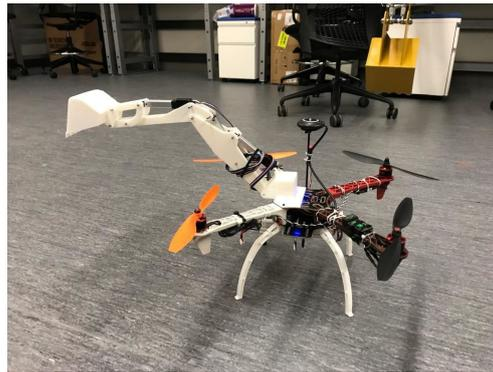
**Figure 1.** The first design of an autonomous flying excavator.
